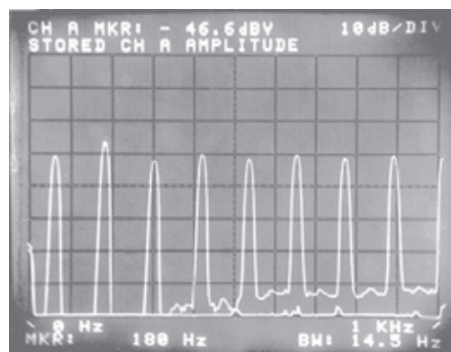
Fig. 1 Noise induced in two-conductor shielded cable (MVVS)
